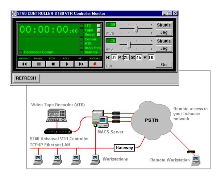
Television stations and cable TV operators frequently use Video Tape Recorders (VTRs) which are installed outside studios and control rooms. It is often very inconvenient for the technicians to walk into another room to operate a VTR. *Micus Alarm and Control System (MACS)* provides a simple solution to that problem – remote access to one or more VTRs from any computer workstation in the studio or in the control room, using the ST60 universal VTR controller from DNF Controls.
